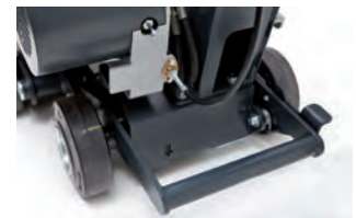
Foot lever for transport position = fast machine relocation
